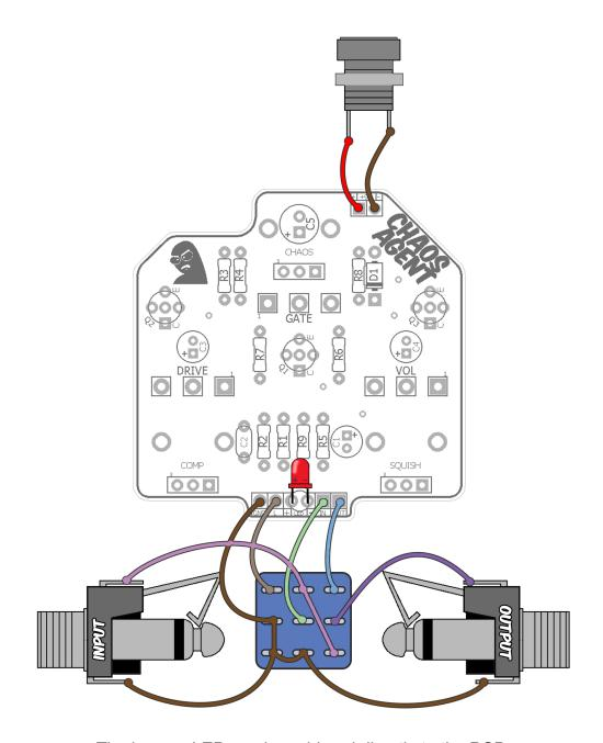
The bypass LED can be soldered directly to the PCB.
