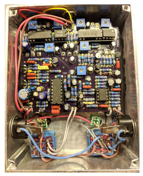
This prototype design is very old. I think I did it around 2013 and did not get around to completing it until 2018. It includes modulation with an AQB\_MOD board mounted under the main PCB. Since this was a pretty big hassle, I ended designing two versions of the Man O War - with and without modulation.
