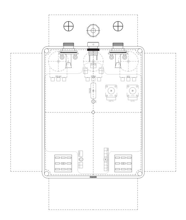
The two LED bypass indicators (effect bypass and Tails bypass) as well as the modulation LED (LED3) should be soldered directly to the PCB. Place them loose in their pads. After mounting the PCB in your enclosure, move the LEDs into place in their respective holes and solder in place.
