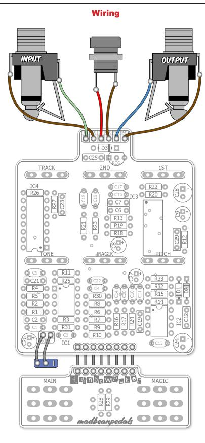
An 8-pin, 1" ribbon cable is recommended for soldering the connections between the two PCBs.
