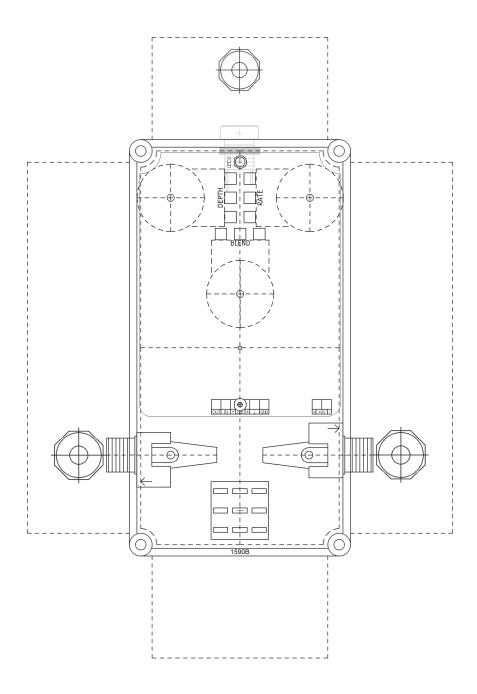
I recommend using the smaller Lumberg style jacks for the input, output and DC jacks on this build. It's a tight fit in the 1590B.
