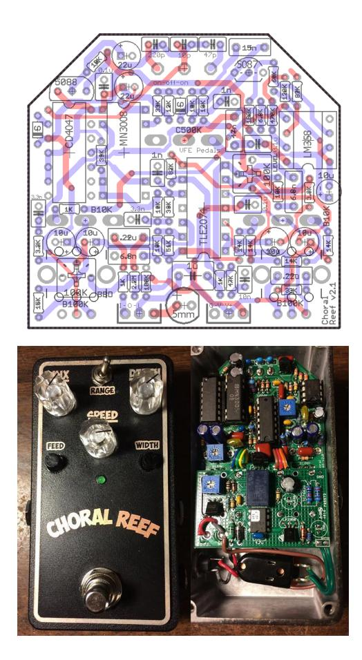
Note: I used a small profile electrolytic in place of the 10uF tantalum cap.
