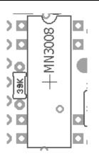
The audio board indicates a 39k resistor right under the MN3008. I suggest installing this resistor on the bottom of the PCB and using a socket for the MN3008.
