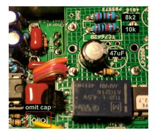
On the audio board, do not populate the area labeled "omit cap", This capacitor is not listed on the schematic or BOM.
