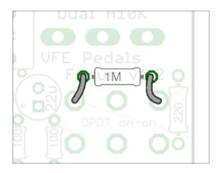
PS: Insofar as I can tell, there is not real difference in v1.1, 1.2, or 1.3 of the PCB other than this 1M resistor. He may have done small tweaks on the trace routing or values but the values listed in the BOM are for the last version, which is 1.3.
