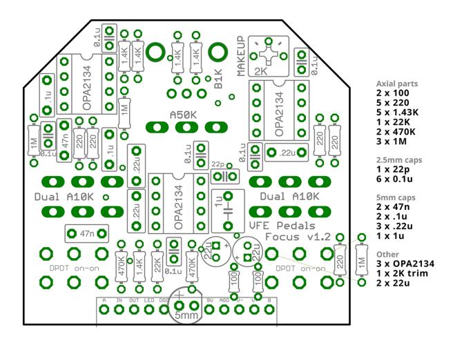
Note: Use the values listed on the image above – not the values indicated on the silk-screen of the PCB. Some values changed over time in the VFE product cycles.
