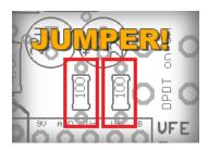
Version 1.1 of the Focus (the board that ships with this project) requires a 1M resistor soldered across the two outside pins of the right-side DPDT. This was added to prevent a small switch pop. Ver. 1.3 (the one shown on the Trace layout on pg.2) has this resistor on the PCB.
