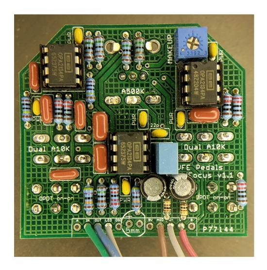
This pic was taken before adding the 1M jumper across the DPDT (right under the "Focus v1.1" text). Also, the 100R resistors are on the PCB because I elected to short them on the bottom rather than remove them (to lessen the chance of damaging it).
