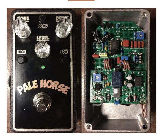
Note: I used two 4u7 BP caps in parallel in place of the 10uF BP.
