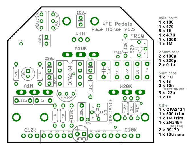
Note: 10kA level pot on the PCB is actually 50kA.
