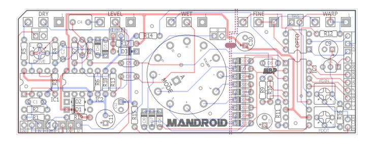
Due to the split-rail power scheme, this project requires an isolated 9v supply. Daisy-chained supplies (ex. One Spot using multiple taps) will not work for the Mandroid.
