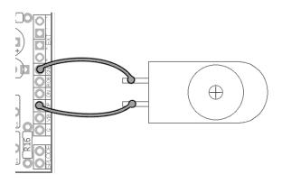
2) Wire up another momentary footswitch. One connection goes to GND (ground) and the other goes to either the UP or DN pads. The ROB pad is not used at all in this project, btw.
