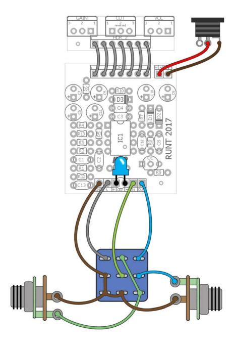
The indicator LED should be wired to the PCB, not mounted directly. LED location shown on the Drill Guide.
