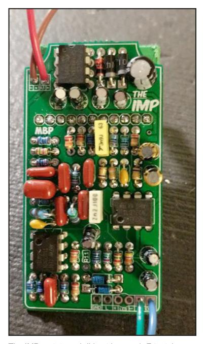
The IMP prototype. I did not have a 1uF tantalum when doing this build so I just used electrolytic. This cap is not in the *direct* audio path so its effect should be negligible.
