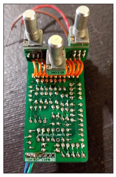
For the final design, I had to change the placement of the three 9mm pots. The dual-gang is longer as you can see above!
