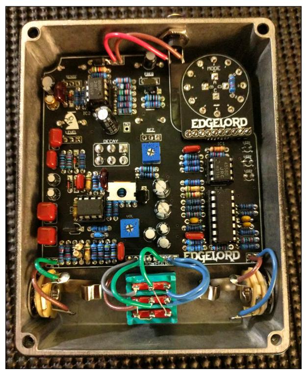
If you use the LM317 (220 style regulator) gently bend the tab to a right angle to allow for clearance on the bottom lid.
