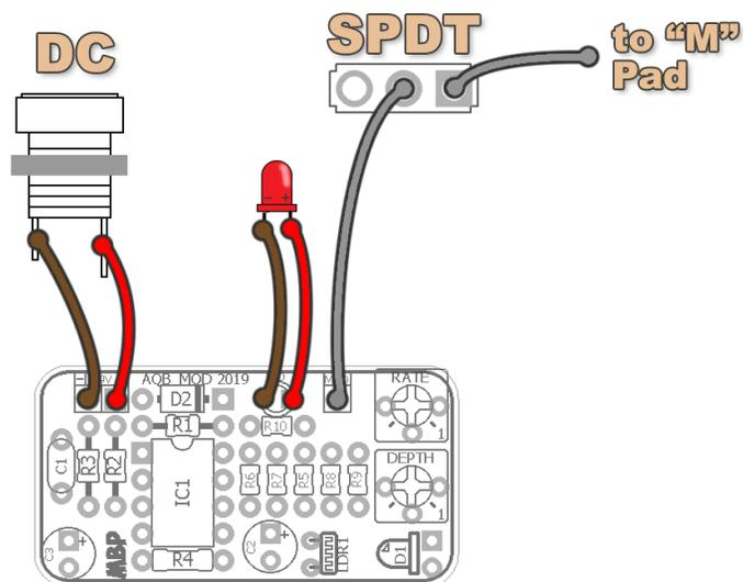
This wiring shows the pots using trimmers. Use this if you only want fixed modulation with the delay.
