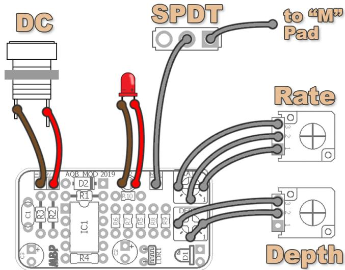
This wiring shows external pots, SPDT switch to turn the modulation on and off and external LED that flashes in time with the Rate setting. Connect the wire from the SPDT to the "M" pad on the Aquaboy.
