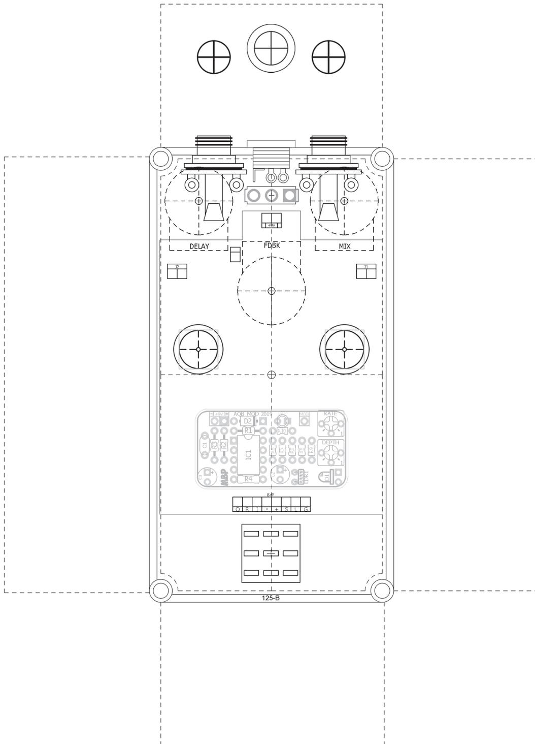
The AQB\_MOD board has to fit under the Aquaboy PCB. Use some 3m foam tape to securely affix it to the enclosure. You could also use velcro!
