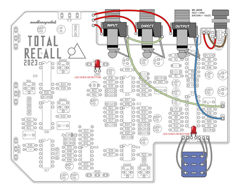
For simplicity, this diagram shows the DC Jack wired just like a negative ground circuit. But, in this case all the red wires are ground and the brown wire is -18vDC. Remember, you must use an isolated 18v supply tap for this positive ground circuit!
