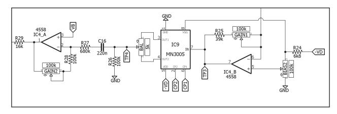
The gain recovery stage starts at IC4\_B. It is fed through an inverted gain stage with a trimmer to adjust the output volume. Here the biasing is done differently with the bias voltage applied to the non-inverted input of the op-amp. At the outputs, we have a new trimmer, BAL. This trimmer is used to align the two output waveforms for minimum phase cancellation and minimal clock bleed. After the BAL trimmer the signal gets sent to the second and final gain recovery stage.
