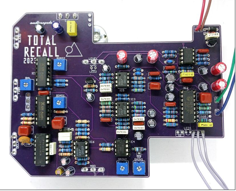
Unfortunately, I only had a ceramic 240pF at the time for this build. I plan on replacing it with a MICA before boxing it up.
