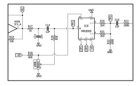
Our audio source comes in at C14 and goes to pin7 of IC8. BIAS1 is our voltage divider also connected to pin7. CP1 and CP2 are the two clock signals, pins1 and 5 are ground and power resp., pin8 is the Vgg voltage (in this case it is set to -14vDC) and our outputs come from pins 3 and 4. These are mixed with another voltage divider created by R41 - R43.
