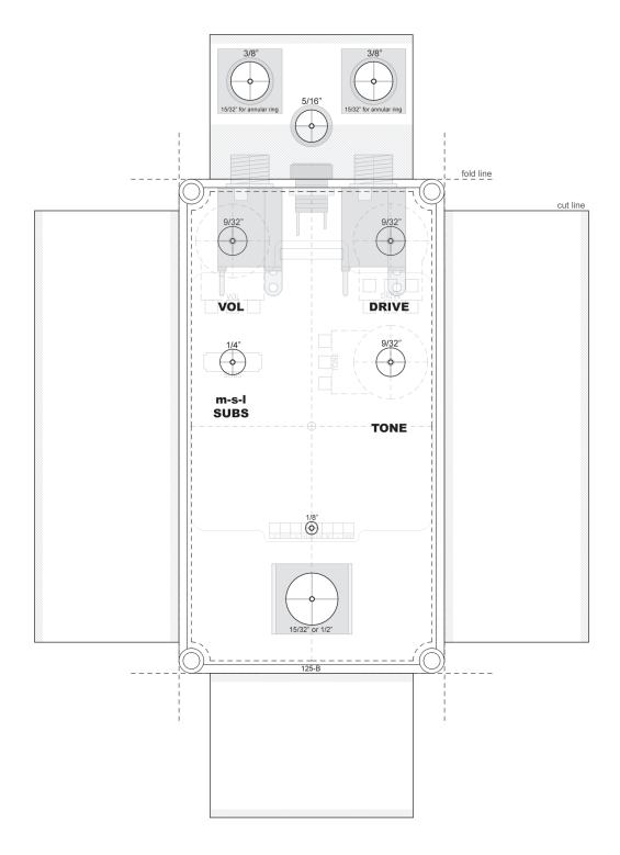
Use this drill template for 3PDT bypass wiring.
