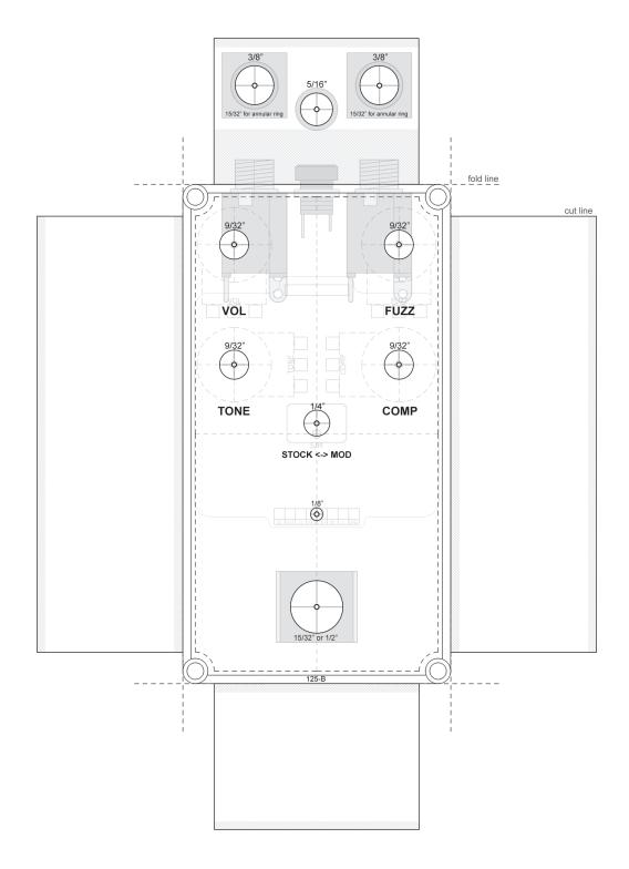
Use this drill template for regular 3PDT bypass.
