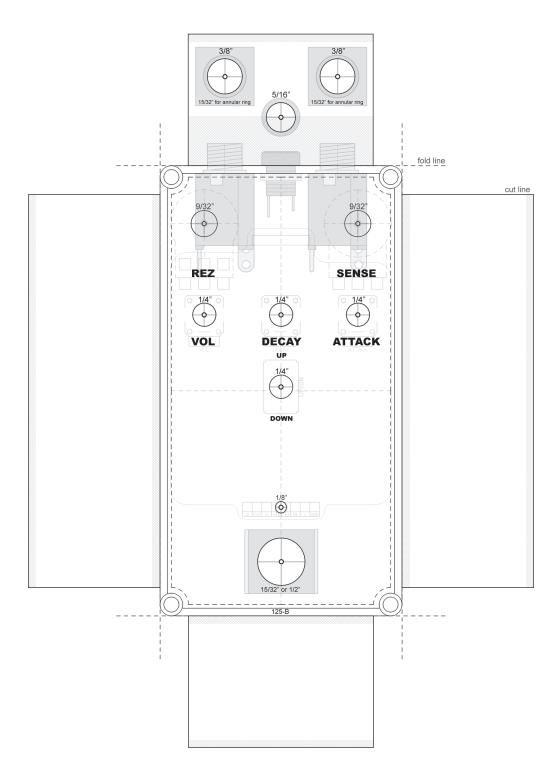
The Batwing is slightly too large to comfortably use any of the Softie bypass boards. I suggest sticking with 3PDT bypass, or using a different relay-based bypass if you prefer.
