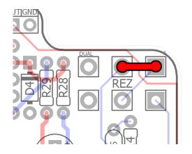
If subbing a single gang pot, solder it to the bottom row of the REZ pot.
