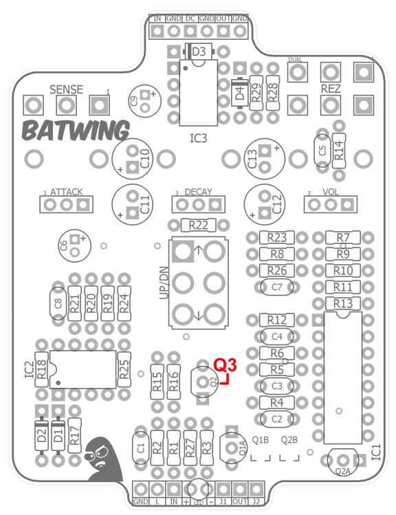
Note: "Q2" is mislabeled on the PCB. It should say Q3. Q2 is a J201 (where Q2a is the through-hole version and Q2b is its surface mount counter-part to give the builder the option of either). **Make sure you put the 2n3906** transistor in the "Q3" spot as shown above.
