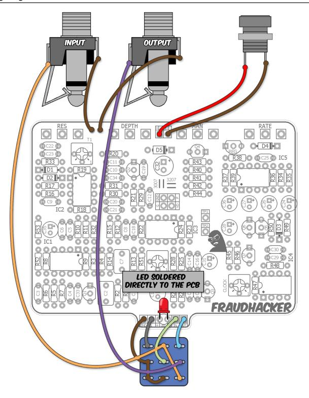
**04.02.23 update:** in the previous version of this doc I advised not to use the "L" pad to wire the LED cathode to the 3PDT and instead use a wire directly from the LED. You do not need to do this. It turns out I had a problem with the specific LED I used in my build (from a cheap batch I bought). You can solder the LED to the PCB as normal and use the wiring diagram above.
