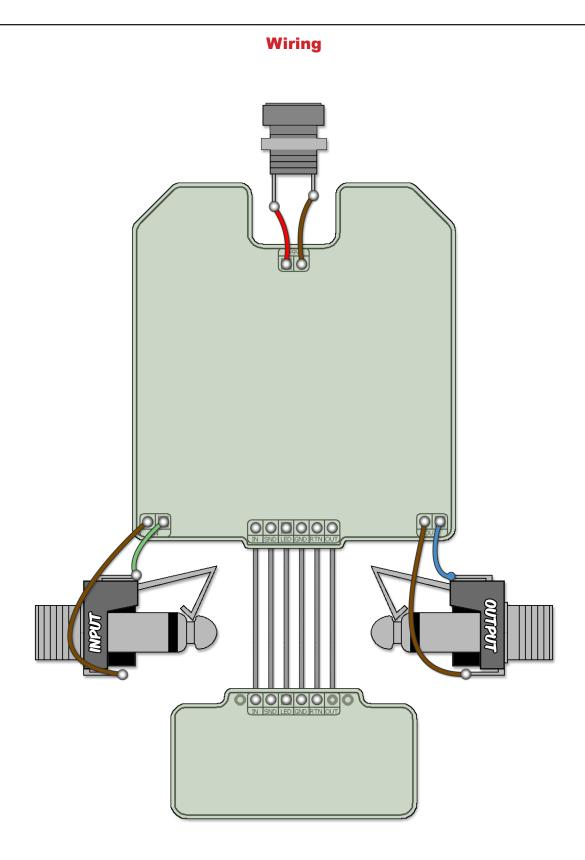
Unless otherwise noted, all Standard Series projects have the same wiring regardless of which 3PDT bypass board is used. A 6-pin, 2" ribbon cable is recommended for soldering the connections between the two PCBs.
