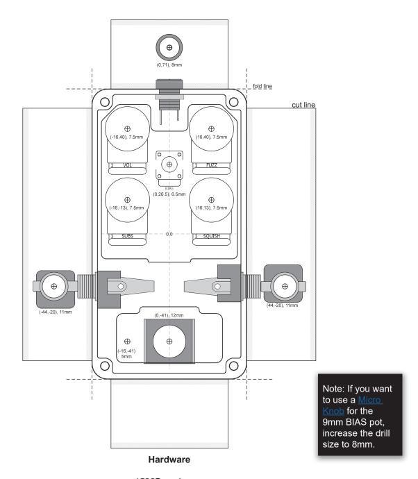
1590B enclosure 16mm pots, 9mm Plastic Shaft pot Lumberg 1/4" Compact mono jacks Slim 2.1mm DC jack Standard 3PDT footswitch
