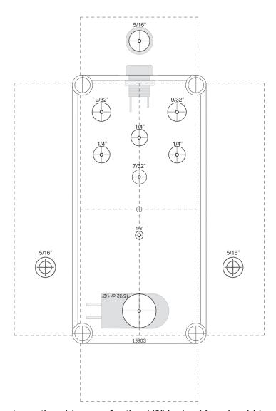
The two drill spots on the sides are for the 1/8" jacks. You should be able to fit a third spot if you plan on using all three possible outputs. **Remember to only drill the spots you need!**
