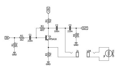
The Magnavibe is a popular DIY Vibrato build (being based on the Tim Escobedo Wobbletron). It would be easy to adapt just the audio portion of the Magnavibe to accept the LDR output of the Tappy, as shown in this example.
