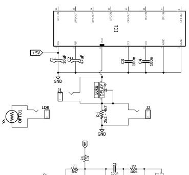
Here's an example of a possible delay modulation controller using a typical PT2399 setup. There are actually two ways you could do it.
