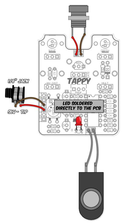
The wiring is the same for all three possible jacks. Just make sure you keep track of tip (square pad) and sleeve (round pad). I don't recommend the mbp mini-jack adapaters in this build since it only requires two wires per jack.
