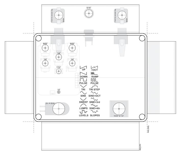
If you want to incorporate the Tappy PCB into an all in one type build here's a 1590BB template to help get you started. You can find the .PSD template in the zip file for this project.
