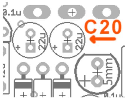
The NE555 is used as a charge pump to create around 22v as the supply on the audio path. A 35v rated 22uF for C20 would be ideal, but if you only have 25v rated caps stick with that. Space is pretty tight in that area.
