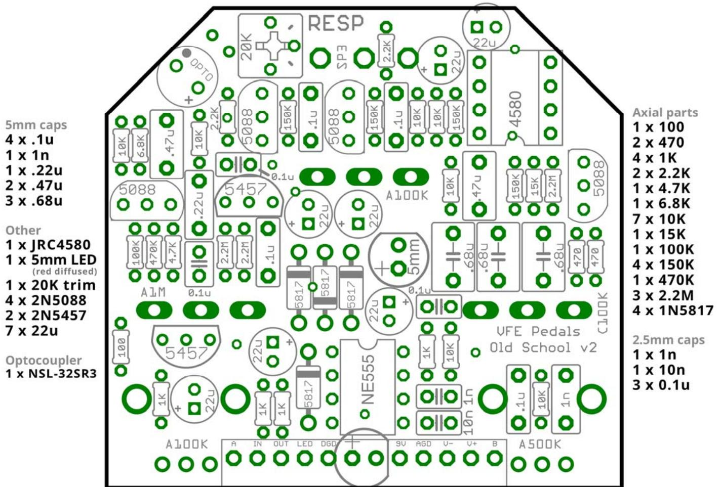
**Note:** Use the values listed on the image above – not the values indicated on the silk-screen of the PCB. Some values changed over time in the VFE product cycles.
