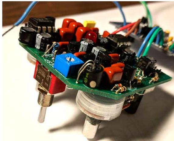
Note how the optocoupler is installed. The dot on the opto corresponds to the dot on the Old School silk screen. In general, all the NSL32 optos have the dot indicating the cathode of the internal LED.
