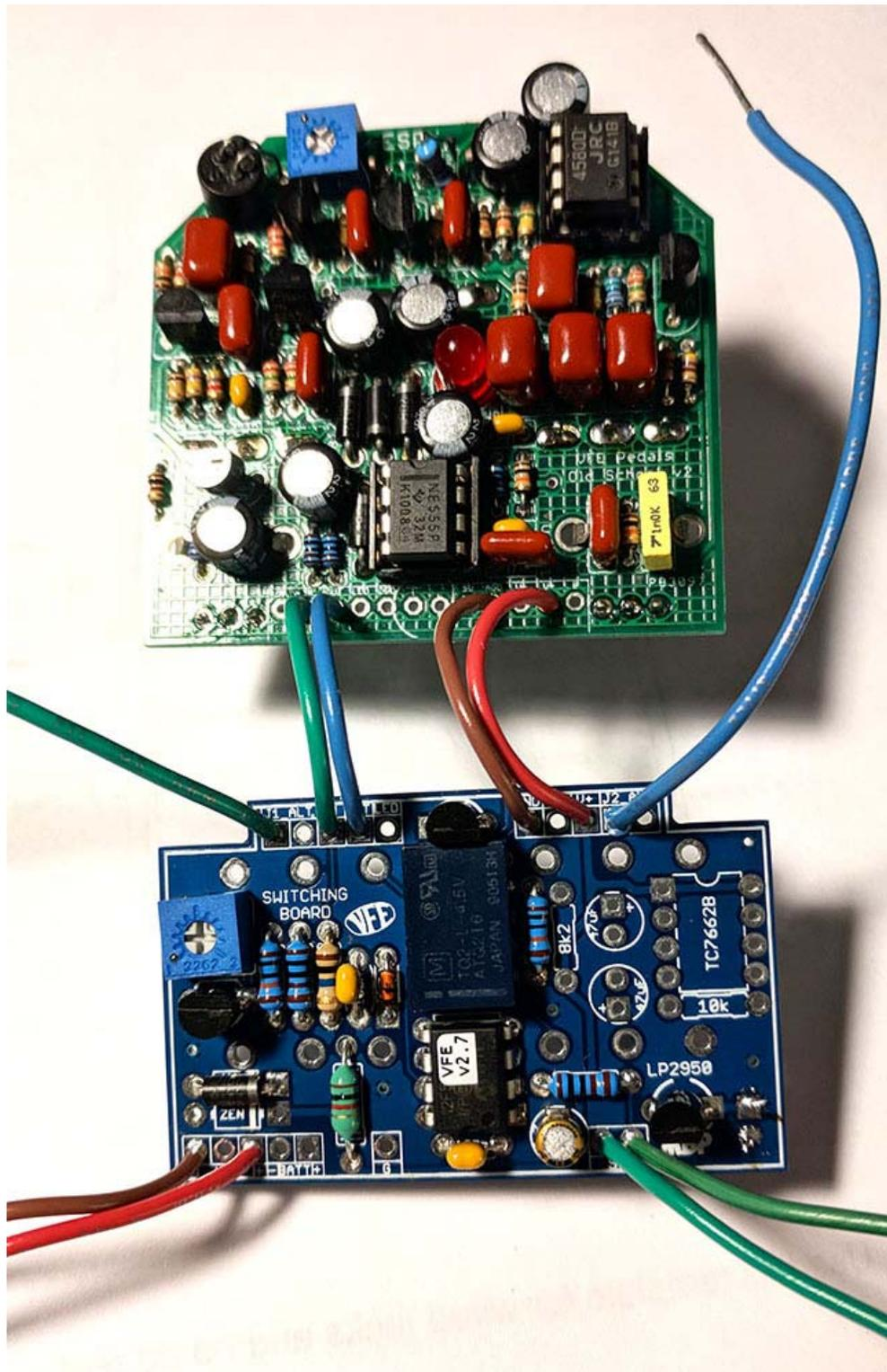
The red LED on the PCB will light up with the speed control, so if you like blinky lights you can wire this LED to the board and make it external on your enclosure for a tempo indicator.
