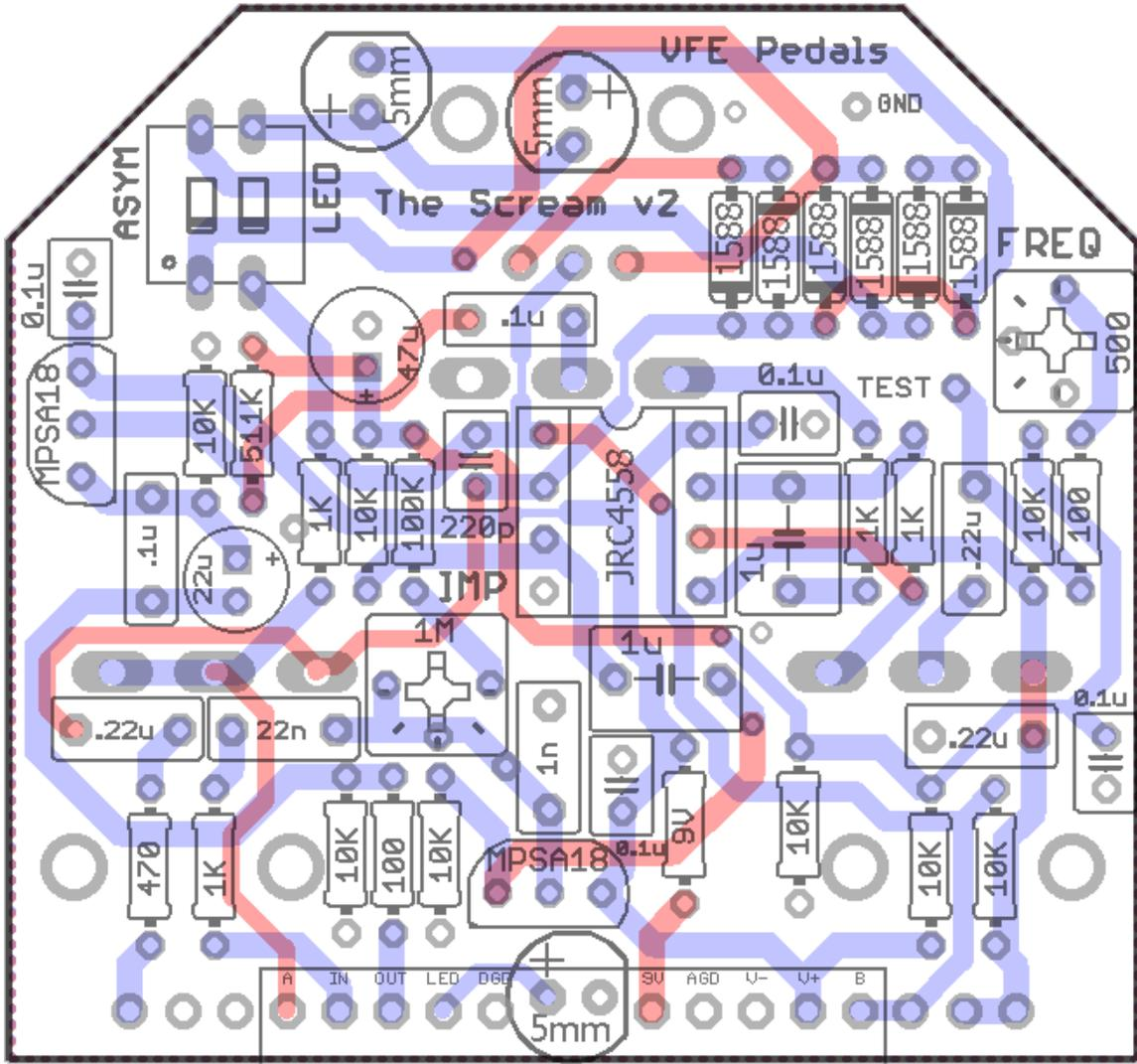
The resistor labeled “9v” should be left empty.
