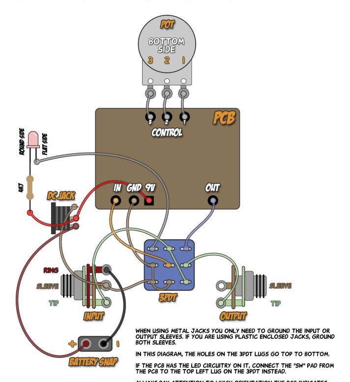
ALWAYS PAY ATTENTION TO WHICH ORIENTATION THE PCB INDICATES FOR THE CONTROL POTS. 3-2-I MEANS THE SHAFT FACES DOWN. I-2-3 MEANS THE SHAFT IS UP (FACING YOU).
