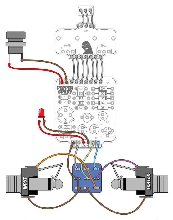
The mini SPDT was intended to be soldered directly to the breakout PCB, but after looking at it again I felt like it was too close to the pots. Luckily there is plenty of room to just wire the switch and give you more space to work the controls.
