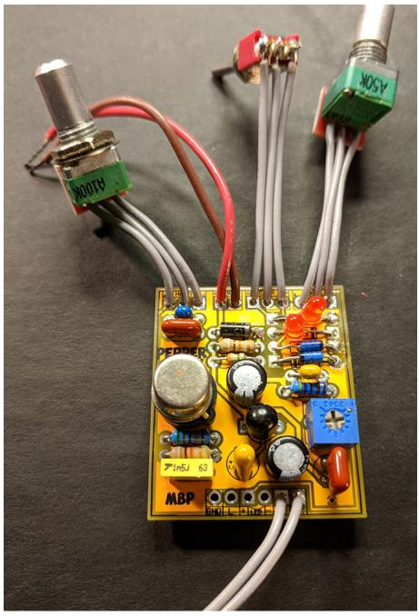
This is the build of the 2018 "giveaway" version of the PepperSpray. The 2019 version adds board-mounted pots on a breakaway PCB and moves a couple caps around (plus fixed one error mentioned in the giveaway version).
