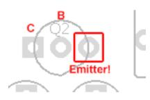
The 2n3565 has a flattened end on the mushroom style casing. The flattened part indicates the emitter. Be sure to put the transistor in the right way!
