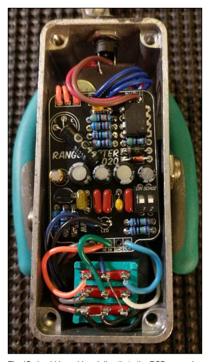
The IC should be soldered directly to the PCB or used with a low-profile 8-pin socket. The standard size socket may be too tall for the 1590A enclosure.
