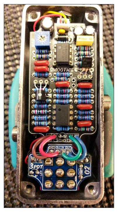
I used low profile 8-pin sockets for the two ICs. I also broke a spare apart to make two 3-pin sockets for the FETs.
