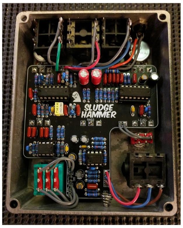
Here's my final build. The board layout changed from 1/8W to 1/4W resistors and resulted in an easier fit for all the hardware. This redesign also allowed me to get it in a 1590BB instead of 125BB.
