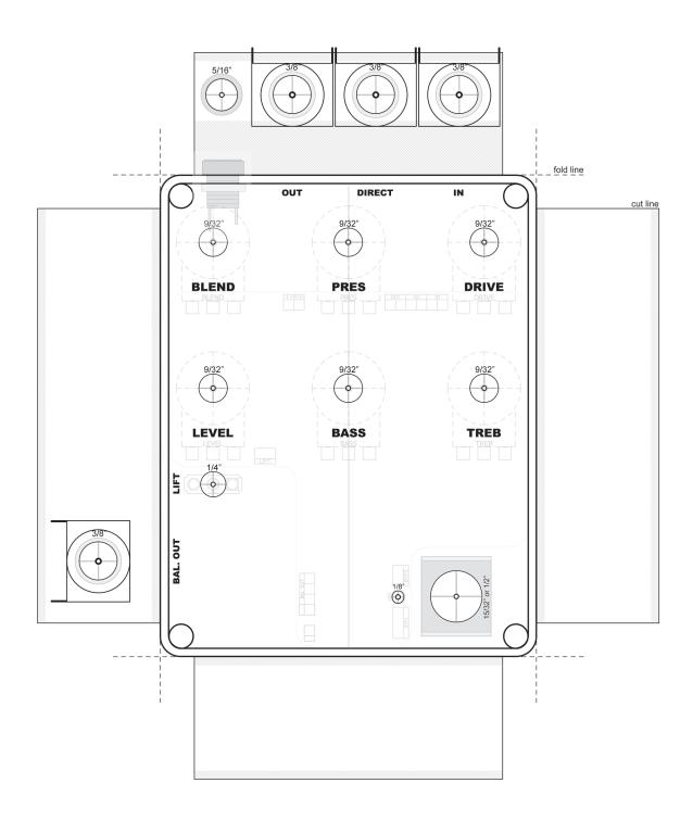
Use this template for all options except when using an XLR. Simply exclude what you do not need. For the Balanced output option, use all drill locations. For no balanced out, omit the SPDT and Bal. Out drills. You can also omit the DirectOut drill if you choose to exclude it. It's a tight fit for the top jacks. Make sure the jack lugs do not contact the bottom lid. Bend the solder lug tabs inward if needed.
