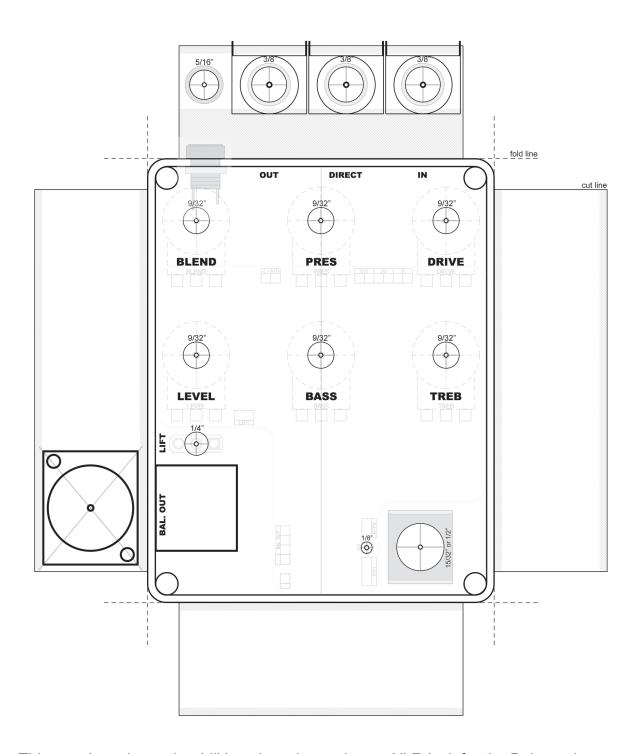
This template shows the drill location when using an XLR jack for the Balanced output. Some may be slightly different in size, but this should cover most. I recommend drilling the large hole first, then place it in the enclosure loose so you can mark the exact location for the screw mounts.
