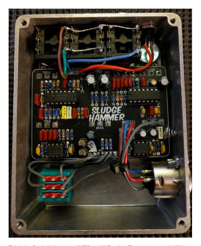
This is the first build. It used a 125BB and XLR option. The board required 1/8W resistors. After this one, I decided to go back to the drawing board to find a better layout.
