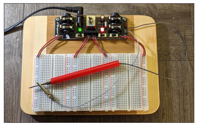
I used a \$5 cutting board from Amazon to mount everything. For the PCB, I used #4 sheet metal screws to secure it to the cutting board. Underneath, I used stick on rubber feet in the corners.
