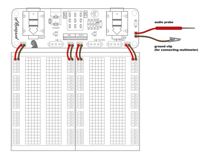
Note the "+" and "-" orientation of the breadboards. The switch is set up to be in effect mode to the right position, and the bypass to the left. **Unfortunately, I put the labels on the wrong way!** If this bother you, just black them out with a Sharpie like I did. I will correct this on the next batch of PCBs.
