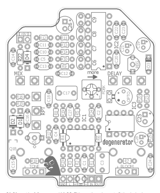
C6-C9 must be 2.5mm spaced MLCC. This was the only way to fit the design in a 1590B. See Notes for suggested parts.
