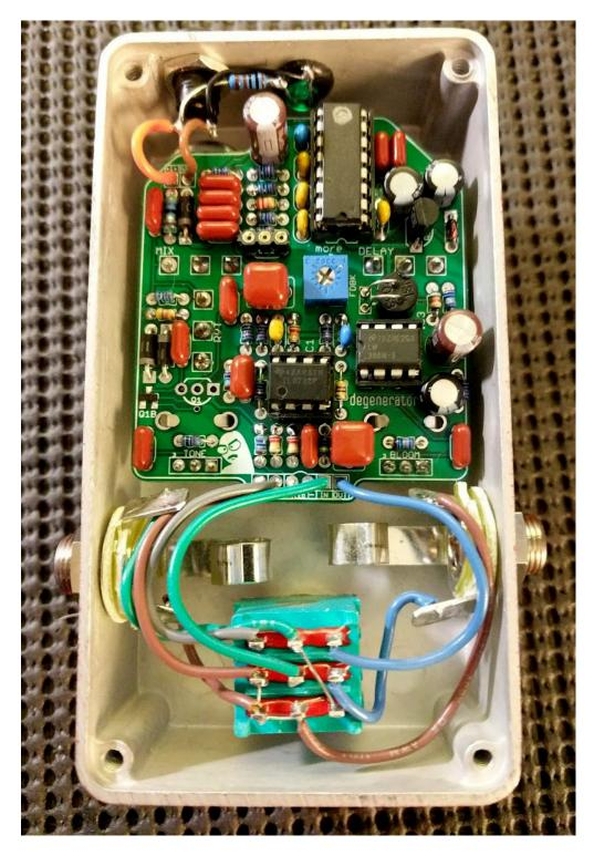
When I drilled the enclosure for my build, I forgot the DC jack needed to be offset. So, I covered the extra hole with a rubber grommet and added a second LED that turns on with power.
