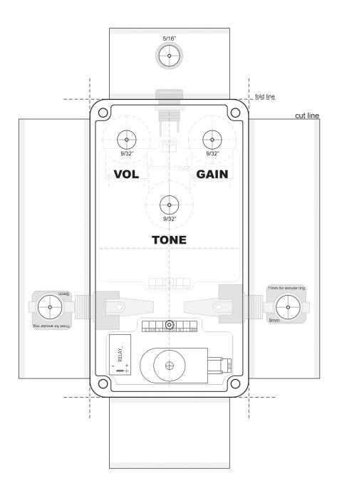
Use this template for "Softie3" relay bypass. Note the different bypass LED location.
