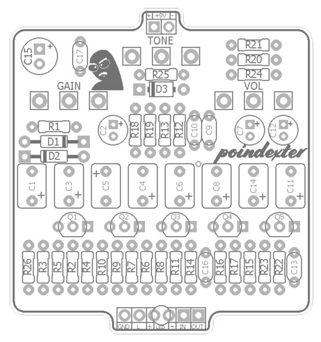
While not on the silk screen of the PCB, I've added a "+" indicator here to denote the positive end of the 10uF caps used in place of film caps. Use this image as a reference when populating your board.
