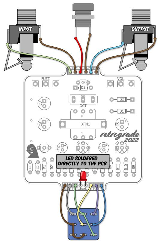
The In and J1 connections were accidentally transposed on the PCB so you will need to follow this diagram for proper bypass.
