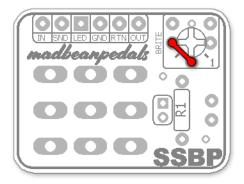
The SSBP grounds the circuit input (SND) on bypass. There is an option to ground the circuit output (RTN) on bypass as well. Generally this is not needed, but if you have an effect that has an unruly "pop" when switched, try the RTN grounding. To enable this feature, solder a jumper wire between the two pads shown below. Otherwise, leave them unconnected.
