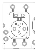
Opto1 has solder pads for both the VTL5C9 and NSL32. I recommend using the 5C9. It is a more expensive parts, however, having tested both devices in this build the 5C9 does a better job of pulling out finer detail in some of the more esoteric waveforms in Bank2. If you cannot get the VTL5C9, use the **R3** version of the NSL32.
