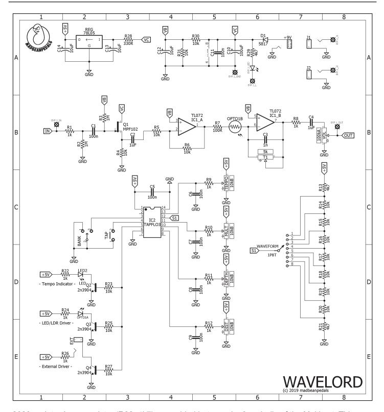
2020 update: A new resistor (R32: 4k7) was added between lug3 and +5v of the Multi pot. This prevents the control from resetting when turned fully clockwise. 2021 update: R28 is now 100R.
