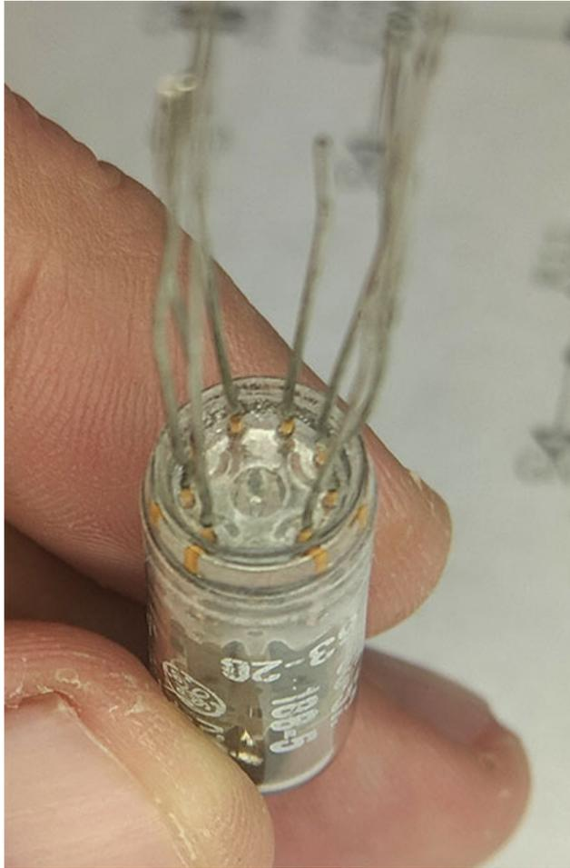
The leads on the tube form a U shape. This tells you the orientation.
