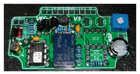
Start by populating your components for the particular switching scheme you need for your VFE build. This is for a single supply circuit so I have left the charge pump and associated electrolytic caps empty. The MCU should be soldered directly to the PCB (as well as charge pump when used) and the three transistors should be bent slightly down after soldering (to clear the bottom lid when in the enclosure).
