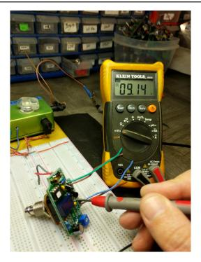
Before hooking up the switching board to any VFE PCB, it's a good idea to first do a couple of simple tests. Power it up on a breadboard and press the momentary switch. You should hear a soft click from the relay as it toggles.
