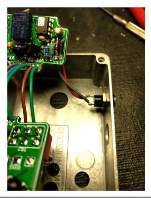
After you have you have everything wired up and tested, I suggest first soldering the wires to the DC jack. This will make it much easier to load everything in. Be sure to leave some extra length on these wires so you have enough room to move things into place in the enclosure.
