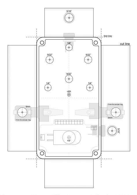
This drill diagram covers ALL current VFE projects except the Fuzz Duo (which has a drill diagram in its project doc). I've shown drill diameters for the Lumberg style 1/4" jacks and a Thinline DC jack. You can use the same drill locations for other styles of jacks (enclosed, metal frame like Neutrik, etc) but their drill sizes will be different.
