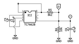
For audio effects that use a split-rail design, a 7662 is used as an inverter. The filtered DC is connected to the 7662 at pin8. Pin1 is shorted to pin8 to utilize the on-board frequency booster. This keeps the internal oscillator of the 7662 out of the audio range. Pin5 outputs a negative voltage (V-) and is decoupled with a 47uF cap (C6). The second 47uF cap (C5) is used to charge up the voltage inversion within the 7662.
