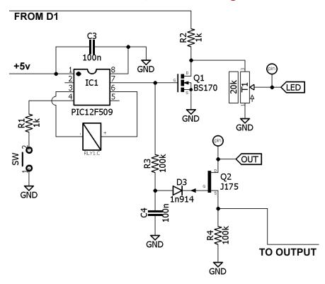
The 5v tap connects to the micro-controller (IC1: PIC12F509) for power. The relay coil (TQ2-L-5v) connects to pins 3 and 6 on the PIC. Pin4 of the PIC connects to ground via a 1k resistor and momentary switch. When the momentary switch is depressed, the PIC "reads" that input and sends a voltage pulse to the relay to activate the coil. This causes the internal DPDT of the relay to flip states (between bypass and effect in our case).
