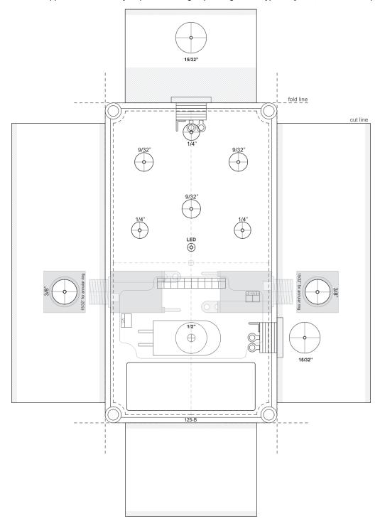
Here is a 125B drill diagram with the option for battery operation. This template has not been tested but everything should fit. Battery wiring is independent of the v3 switching board and should be done directly. If you do use the battery option, I suggest these parts:
