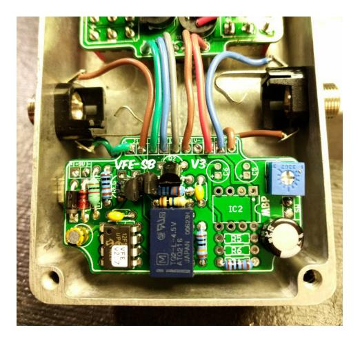
Make sure you leave some room between the bottom wall of the enclosure and the switching board. This will ensure the lip on the bottom lid clears the relay and can sit flush.
