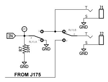
The Switching Board utilizes an effect-input grounding scheme. IOW, when the audio circuit is bypassed its input is grounded. A 10M pull-down is used in all VFE projects.
