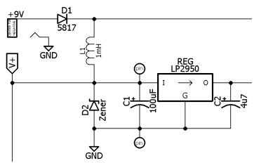
The DC Jack inserts into +9v. Power is reverse-polarity protected via D1. It then passes through a 1mH inductor which creates a low pass filter with the C1 decoupler. This helps reduce noise and minimize ripple on the DC power (additional 100n decoupling caps are used on the audio boards). A Zener diode is included to prevent over-voltage to both the audio PCB and the 7662 inverter (when used). The Zener value depends on which audio circuit is being built.
