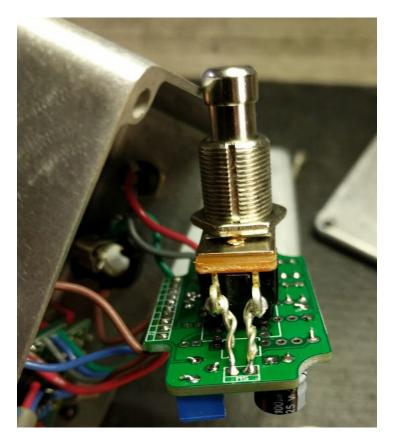
For the switch, I used some 22AWG bus wire and twisted it a bit for extra strength. This holds the momentary switch and switching board firmly in place. But, you don't need to run out and buy bus wire for this. You can use regular wire. All the wiring to this board will help keep it in place plus the enclosure lid will add a slight amount of downward pressure. Use a couple strips of double-sided tape between the board and switch as an alternative.
