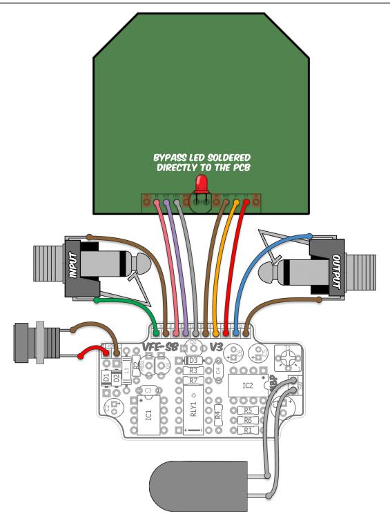
The wiring shown is used for all split rail circuits (IOW, when the effect uses both +9v and -9v). For single supply rail (+9v only such as the FuzzDuo, Distoriton3, AlphaDog, etc) the same wiring is used except <u>you will not wire</u> the V- pads on the switching board or VFE PCB (orange wire).
